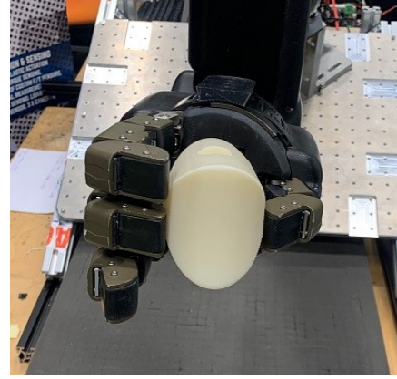
Fig. 1. Three fingers grasp performed during the experiments of the proposed grasp planner. The experiments have been conducted with HERI II Hand mounted on a robotic arm.
